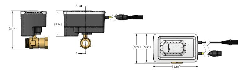
Meter cable shown above is an option for the AquaFlow valve when reading a meter is desired. Specifications are subject to change at the sole discretion of Aquana, LLC.
